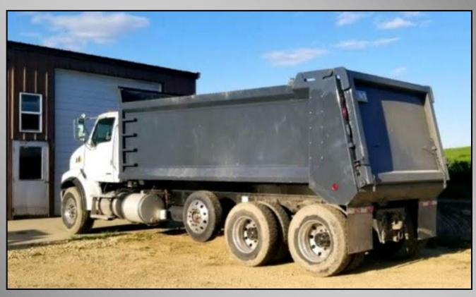
The Kann steel dump body features standard 3/16" Hardox 450 structural steel walls, a 1/4" Hordox 450 floor and weighs about 6,000 lbs. (i.e. ~300 lbs. per liner foot of body).
